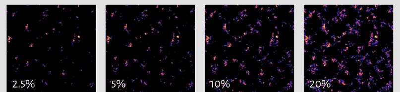
BE simulations of the qualitative evolution of contact pressure for increasing normal load. The ratio of real contact area to apparent contact area is indicated.
